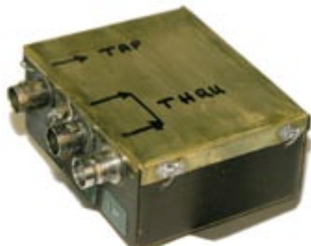
Figure 2 — Sample of a box made with PC board with a sheet brass cover overlapping all four sides. Note the BNC connectors and feed through insulator.
