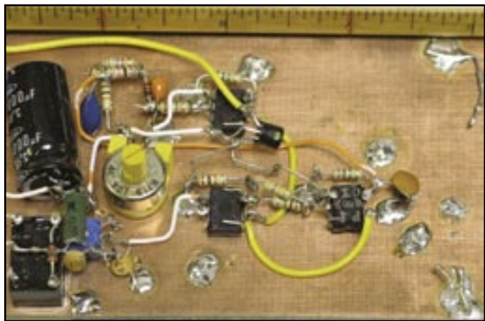
Figure 3 — Sample of "ugly construction" method.
